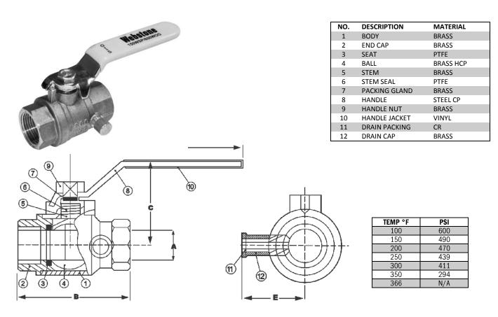
**Specifications:** Designed for residential, commercial or industrial use with water, oil or gas. This approved Webstone valve is actuated by a blowout proof stem and features an adjustable packing gland. Threaded ends comply with ANSI B1.20.1
