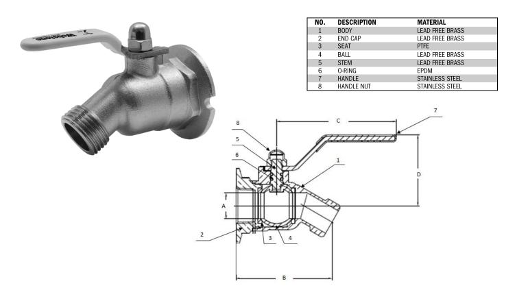
**Specifications:** Designed for residential, commercial or industrial use with water, oil or gas. This approved Webstone valve is actuated by a blowout proof stem and features an adjustable packing gland. Threaded ends comply with ANSI B1.20.1
