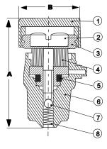
**Specifications:** Designed for residential and commercial heating applications for use in hot water baseboard. Allows bleeding of air from the system and protests the system from damage due to thermal expansion because of the spring loaded ball design. These valves provide manual or automatic air venting in radiators, convectors, baseboards or high points in piping systems. Ideal for hot water and low pressure steam systems.
