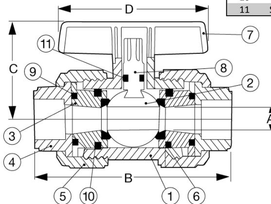
**Specifications:** Designed for residential or commercial use with water. This approved Webstone valve is actuated by a blowout proof stem. Not for use with potable water. Threaded ends comply with ANSI B1.20.1
